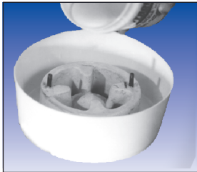
Pouring Replicast Around a Model
